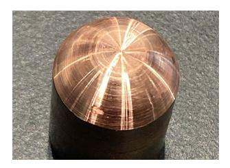
\*Figure above shows the chip after repeated push-up motions. Radial marks can be confirmed.
